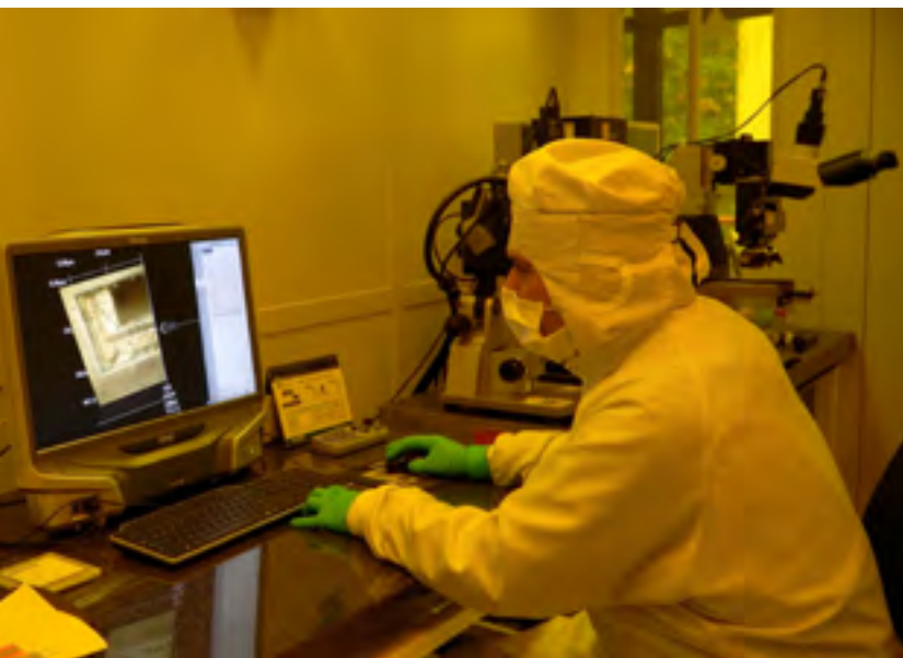
Microscopic 3D analysis of a photo-lithographically produced structure in the clean room of the Centre for Semiconductor Technology and Opto-Electronics.
