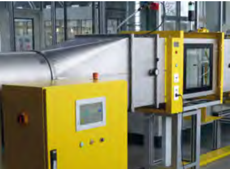
Versuchsanlage zur Untersuchung raumluftechnischer Filter Pilot plant for the investigation of room-air filters
